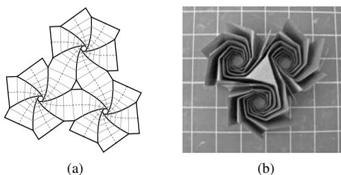
FIGURE 2. (a) Crease pattern and (b) paper demonstration of the hexagonal-spiral fold architecture.
