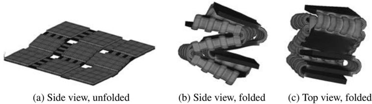
FIGURE 6. Final configuration of the Miura-fold system with nine angled rigid plates connected by hinges, as simulated in ANSYS.
