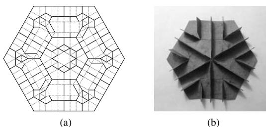
FIGURE 3. (a) Crease pattern and (b) paper demonstration of the hexagonal-radial fold architecture.
