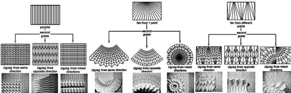
FIGURE 16. Second grade division of accordion patterns.
