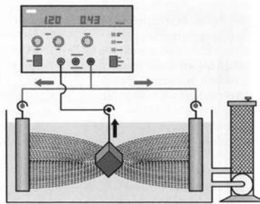
FIGURE 4. The electroforming process [Curtis 04].
