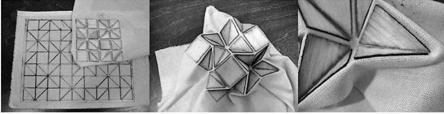
FIGURE 20. One of the first samples for a model-making material: laser-cut veneer glued on textile.
