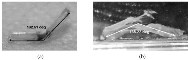
FIGURE 8. Manufactured two-rigid-plate system (a) before actuation of folding and (b) after actuation of folding.
