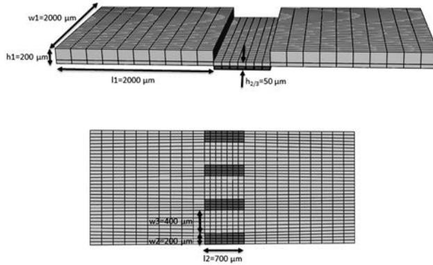
FIGURE 4. Two-rigid-plate system prior to folding, showing structure meshed in Abaqus.
