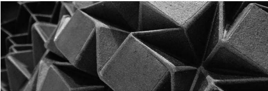
FIGURE 5. Electroformed platelets on textile, with bare fabric hinges.
