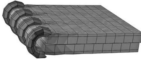
FIGURE 5. Final configuration of the folded two-rigid-plate system simulated in Abaqus.
