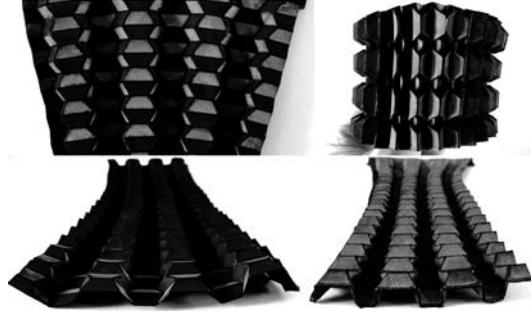
FIGURE 13. By coloring half the platelets, the material seems to change color when seen from different angles.
