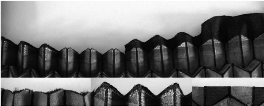
FIGURE 11. Different ways of finishing the edge (top) with close-ups (bottom). Copper on polyester fabric.
