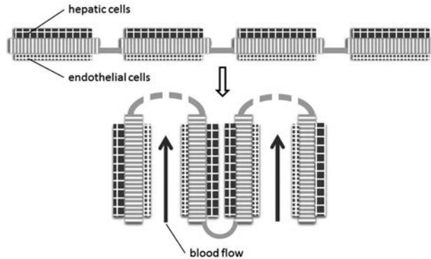
FIGURE 1. Conceptual design of a scaffold, showing a planar scaffold before folding (top) and after folding into three dimensions (bottom). The hinges may be made of the same material as the plates as long as each hinge's thickness and length are chosen to enable the desired folding architecture.
