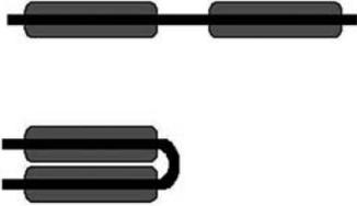
FIGURE 9. The width of the textile hinge is twice the platelet thickness to allow for folding.
