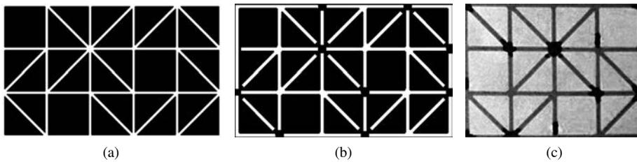
FIGURE 6. (a) Folding pattern is drawn; folding lines are given a certain width. Black areas will be printed in conductive ink, so metal can adhere there. (b) Connections are drawn, so that an electrical current can run through each platelet. (c) Connections are covered with a lacquer to prevent metal from building up in these places.
