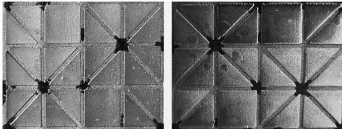
FIGURE 7. The fabric with metal platelets after electroforming, front (left) and back (right).
