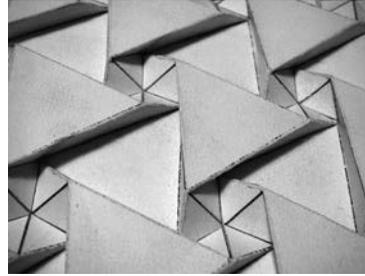
FIGURE 10. The hexagons do not need creases to be folded in paper, but they need hinges in the location of the black lines to be foldable in MFT.
